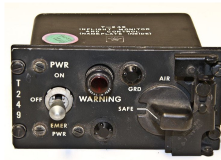
T-249 Arm/Safe Switch. Photo via the National Security Archives [kinda’ looks like our old AMAC Box, doesn’t it? - Ed.]
